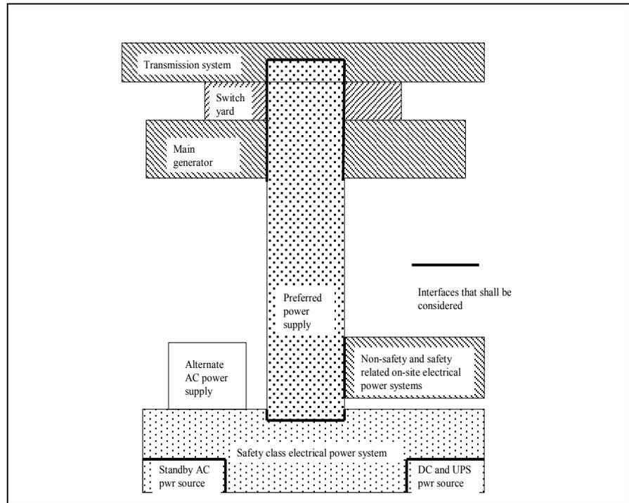
Fig 3 Interfaces to be considered in the analyses (based on IAEA DS 430)
