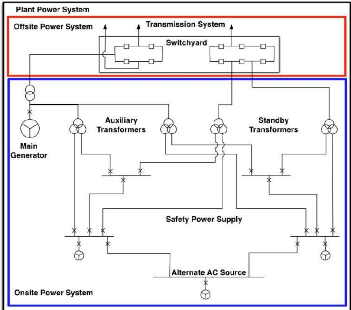
Note This figure is only an example. Various arrangements of buses, loads, generators, and interconnections will meet the requirements of SSR 2/1. Furthermore, many elements of the plant power system, such as buses that are not important to safety, and DC power systems are not shown.
